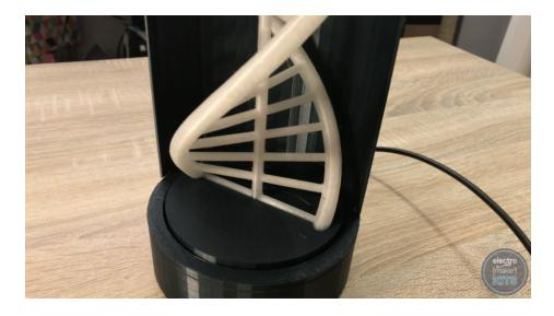
As long as it is well balanced the only thing the 3D printed helix part should come into contact with is the shaft of the stepper motor. If you hear any scraping noises check that the edges of your prints are clean of any stray plastic and that the helix is well balanced.
