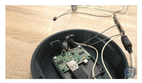
Use more glue to ?x the switch for the LEDs at the top of one of the U shaped columns. The top of the switch should be ?ush with the top of this column. Take care that glue does not prevent the switch mechanism from actually switching.
