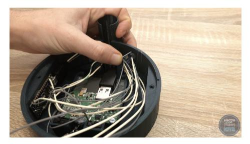
Use another liberal helping of glue to ?x the motor driver into place. I put glue on the bottom of the enclosure and sidewall to hold the driver in position.
