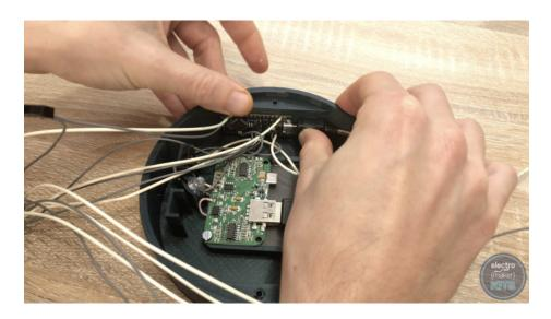
Apply a generous helping of glue to the rear-side of the Arduino and ?x it in place on one side of the enclosure.
