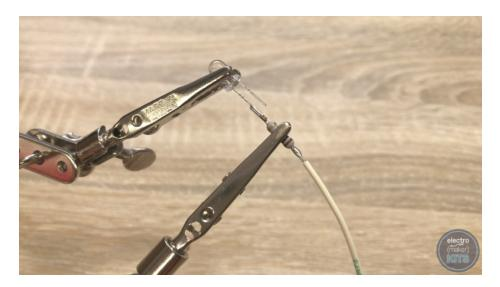
Solder the longer and leg of each LED to each of the two resistors.
