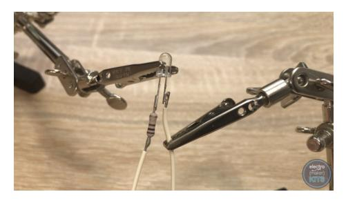
Now prepare two more wires, one 5cm long and the other 12cm long. Solder one to the unused leg of one of the LEDs and repeat with the other LED and wire.
