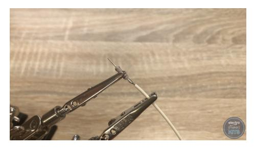
Solder one wire to one resistor and repeat with the other pair.
