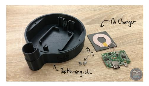
We'll start the assembly by installing the QI charger into the top housing.
