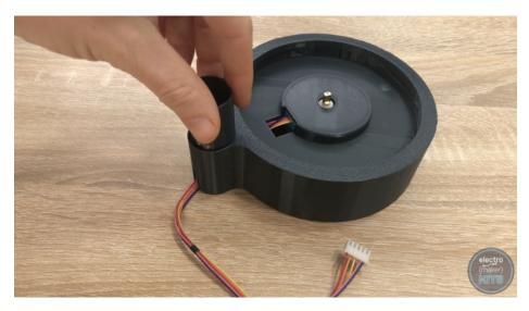
Apply a small dab of glue the outside of the 'Joiner' print and insert this into the assembly we have just been working on. The long rod end is inserted ?rst and the shape of the part will ensure it is inserted in an orientation that will not block any cable runs which we will be using later. Insert it all the way in until the part touches the table.
