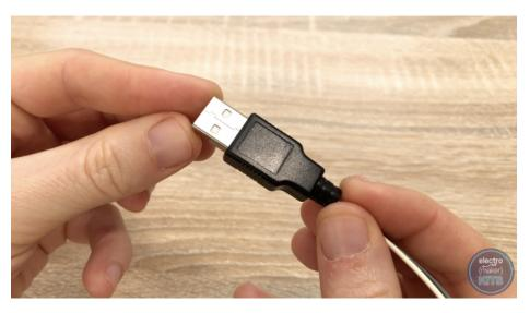
You can then ?nish the assembly of this end of the cable by push ?tting the two plastic halves of the connector around the electronics.
