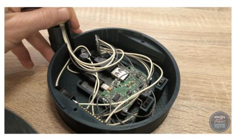
Connect the factory-made USB cable to the QI charger and route the cable through the outlet at the rear of the enclosure. Route the unconnected wire coming from the stepper motor along the same path as well.
