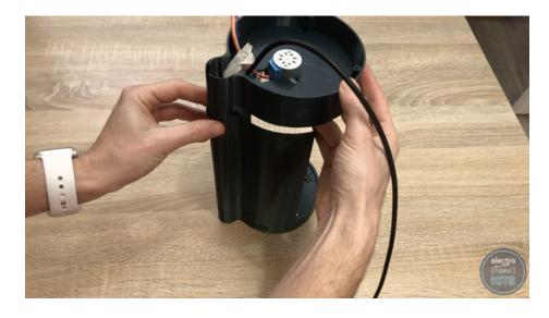
Thread the cable through the tunnel at the rear of the base housing and ?t these parts together.
