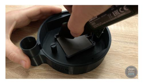
Place the coil face down in its holder and use a few dabs of hot melt glue to keep it in position against the print.
