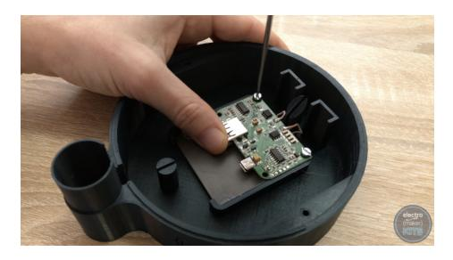
Once the glue has cooled you can fold the circuit board carefully back over the rear of the coil and hold this in position by using two of the M3 x 6 screws in your kit. These need to be done up ?rmly, but be careful not to over tighten them.
