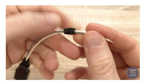
Before we solder the other end you'll need to take the small rubber sleeve from the Micro B connector and thread both the wire through it.
