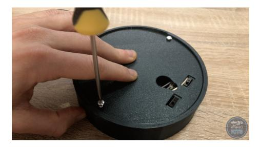
The top cover can then be seated in the enclosure and screwed into place using two of your M3 x 6mm screws.
