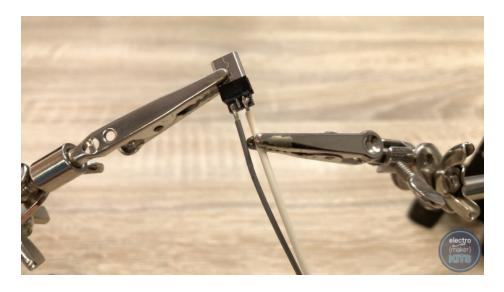
With the micro B plug facing away from us and the side with three pads on it (not the side with two) facing upwards the grey wire is soldered to the left hand side and the white wire to the right hand side.
