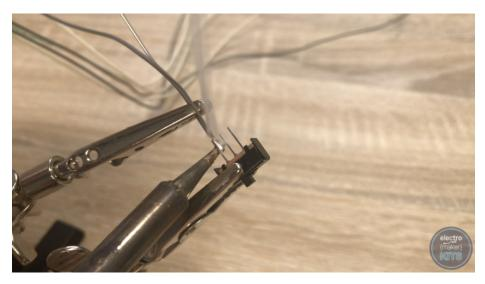
Solder one of the 12cm wires to the positive side of VMOTOR. The other end of the wire is soldered to one of the outside legs on the switch.
