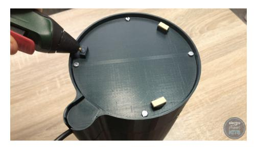
To help reduce noise from vibrations, cut three small lengths of a rubber band and glue these to the three feet.
