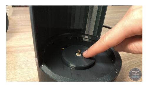
The double helix that we printed earlier is added to the shaft of the stepper motor by aligning the shape on the bottom of the 3D print with the shaft itself. It will only ?t when the two are parallel.
