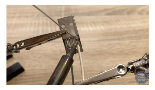
With the pins of the Type A connector facing you and the USB plug away from you solder the grey wire to the pad on the left and the white wire to rightmost pad.
