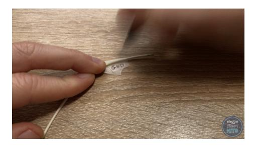
Then use some masking tape or similar to label the other end of each wire. This will make it a lot easier to connect it to the stepper motor towards the end of this project.
