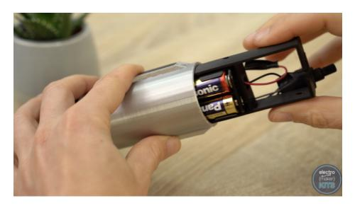
Once it is partway in the roatry switch can be inserted into the end hole from inside the sled (so that the control knob is facing out of the handle). Ensure that the notch on the rotary switch aligns with the notch in the sled.
