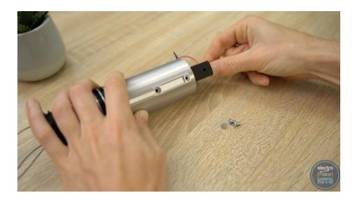
We can then use the four M3x6 screws to hold it into place. Do not use different screws or overtighten them as we don't want to risk damaging the batteries.
