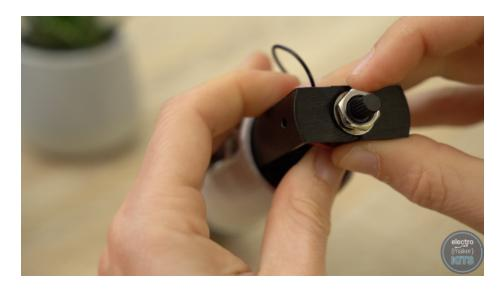
Rotate the sled so that the holes in its side align with the screw holes on the outside of the handle. It can then be carefully inserted whilst being mindful of not trapping any wires.
