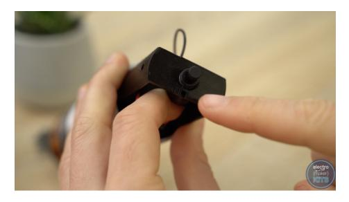
You can then add the washer and nut on the outside and screw down firmly (but not tight) to hold it in place.
