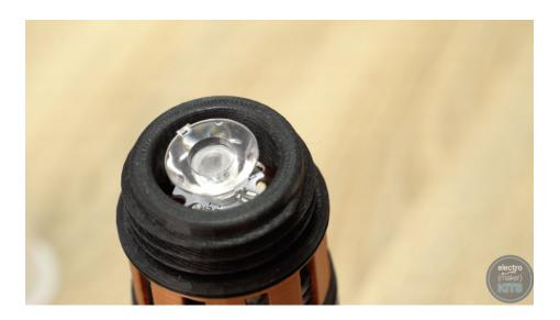
The 3D printed spacer then sits on top of this with the notches in the print face down onto the matching notches on the lens.
