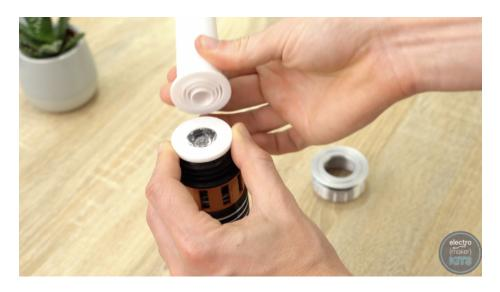
Then the screw top is added over the top of the blades and firmly screwed onto the handle holding the assembly together.
