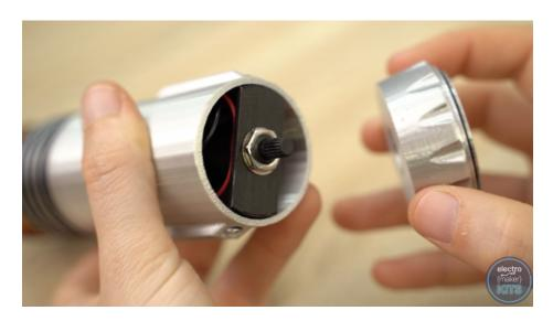
You should then be able to twist it to toggle through the different colours of the LED.
