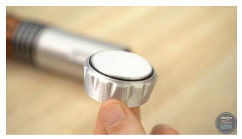
Once the print is complete, remove any support material and push-fit it onto the rotary switch.
