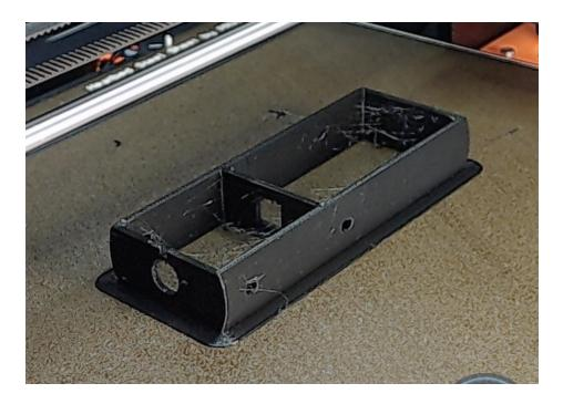
The second part to print holds the battery case in place and provides us with a surface to mount the rotary switch to later. The file is called 'Hilt - Shuttle.stl'. I printed this with a 0.15mm layer height and brim as before. I chose to print it in black as this part can be glimpsed in the finished project at certain angles.
