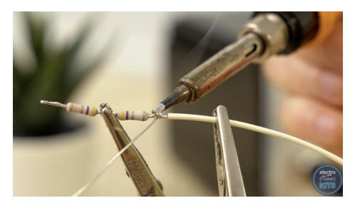
The other side of the resistors is then connected to the 2.5cm wire which you have already attached to the anode on the LED.
