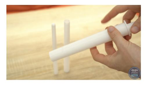
The top end of the hilt is printed almost the same as the bottom end but without the need for supports. I used two different colour filaments, no brim, and no support.
