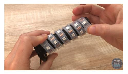
Once you know how far you'll space them they can be unravelled and then wrapped around the column again but this time apply glue as you go making sure each bit has cured before moving onto the section.
