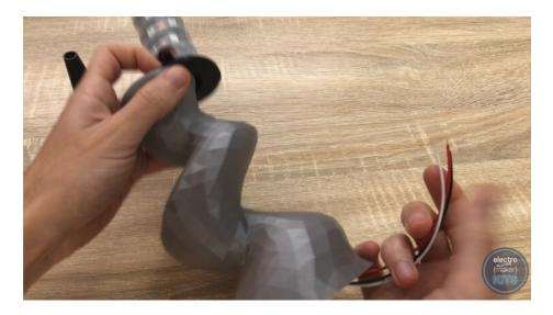
Apply some glue around the rim at the top of the stem and then position the LED holder centrally over the rim and push firmly together whilst the glue sets.
