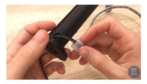
Before we apply any glue it is a good idea to wrap the LEDs around the column so you get an idea of how far apart they need to be spaced before you start gluing them in place.
