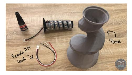
Connect the Female JST connector to the end of the LED wire (they just push together).
