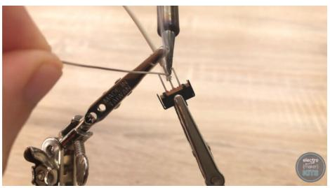
Take the red wire coming from our LEDs (this is the 5v power connection) and solder this to one of the unused legs on one of the switches.
