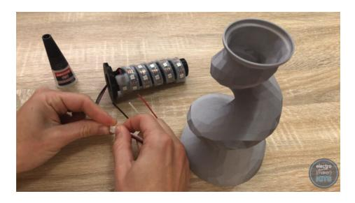
Feed the extended wires down though the narrowest end of the stem and pull them out through the wider end.
