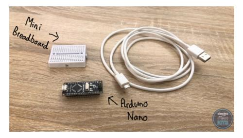
Add the Arduino Nano onto the top of the breadboard and connect the USB cable to it and the other end into your PC. Open the Arduino IDE on your PC. If you have not yet installed this, you can find the free download and instruction here: https://www.arduino.cc/en/main/software
