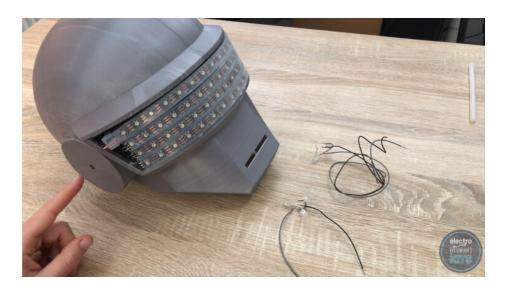
Thread the wires for the LEDs through the hole on the side, then use plenty of glue to hold the LEDs in place as close to the center of the ear as you can. It's also beneficial to keep them pointing away from each other in a triangular fashion if you can so that they can light the ear up uniformly. Don't worry about using to much glue as this area of the ear will not be visible later.
