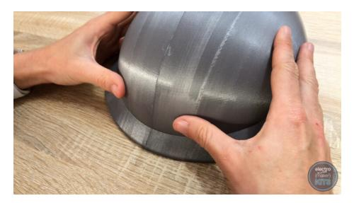
Now we can take the middle section of the helmet, carefully remove the brims and support material from the print and then glue this to the top two pieces we have just been working on.
