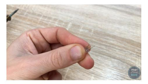
Solder the two negative (shortest) legs together as shown below.
