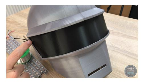
• To comfortably fit all four strip the top one needs to be nestled up as high as possible when installing it.
