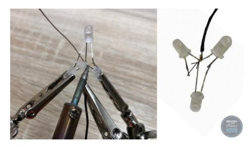
Add a short length of wire to the unconnected positive leg or the trimmed LED to join it to the two other positive legs which are already soldered together.
