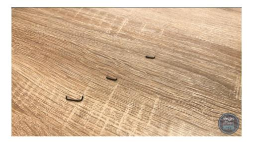
Now you need to solder them at the ends of the LED's where our strips double back on themselves. The contacts are labelled as either '5V', 'DIN' or 'GND'. We need to solder like to like using the 'U" shaped bits of wire.
