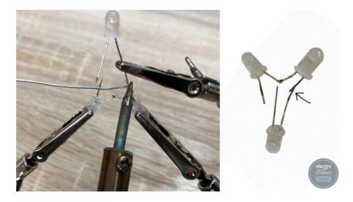
The negative leg of the untrimmed LED can then be soldered to the two other negative legs we soldered together earlier. You may need to bend one or more of the legs already soldered to accommodate this.
