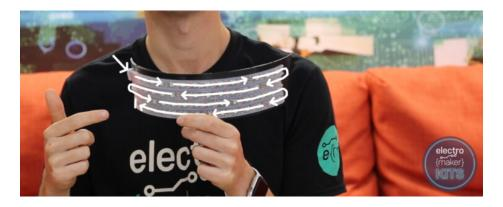
Once you have finished glueing the strips in place you can tuck the three wires through their hole in the top left of the visor.
