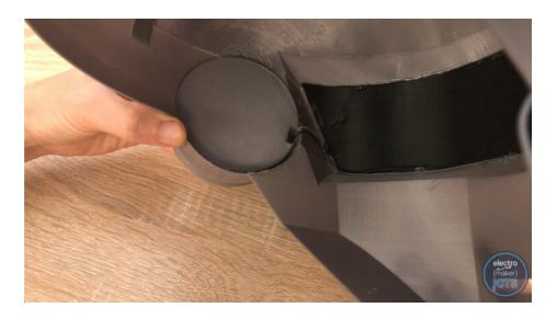
Apply glue to the back of the battery holder and fix this to the battery base we just fitted. Ensure that the end where the wires leave the battery holder is aligned with the wire from the LEDs as we will then glue the battery wires along the same route as the LED wires.
