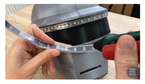
• We need to install the LEDs so that the arrows showing the flow of data through them go back and forth in a zigzag pattern as shown below:
