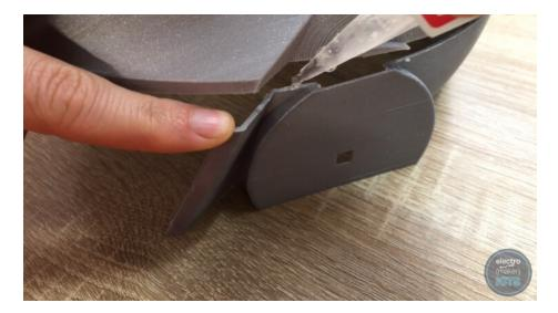
Now turning our attention to the mouthpiece, remove the support structures and brim and apply glue along the area to be joined on one side. We do not need to apply glue along the entire length of this piece - only the area near the two ears actually makes contact with the rest of the print.
