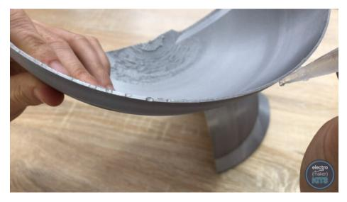
To make this step easier to align I only glued halfway along the joint before holding the two half together. Once this had set I then added glue to the rest of the joint.
