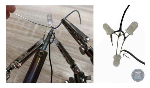
These can be checked quickly by connecting the grey wire to 3.3V on the Arduino via the breadboard it's on, and the black wire to GND (ground). Connect the Arduino Nano to a powered USB port and the LEDs should instantly light up.
