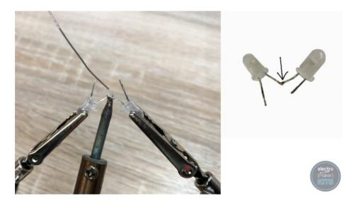
Add a third untrimmed LED by soldering its longest positive leg to one of the long positive legs on the other two trimmed LEDs.
