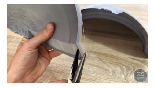
Once removed we can apply dabs of super glue along where the two parts join. Apply the super glue to only one side and then carefully press them together.
